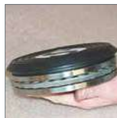
Ball bearing for turning plate
