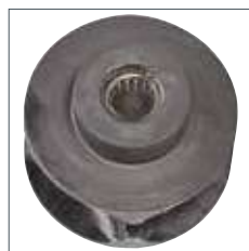
Load chain sheave with needle bearing
