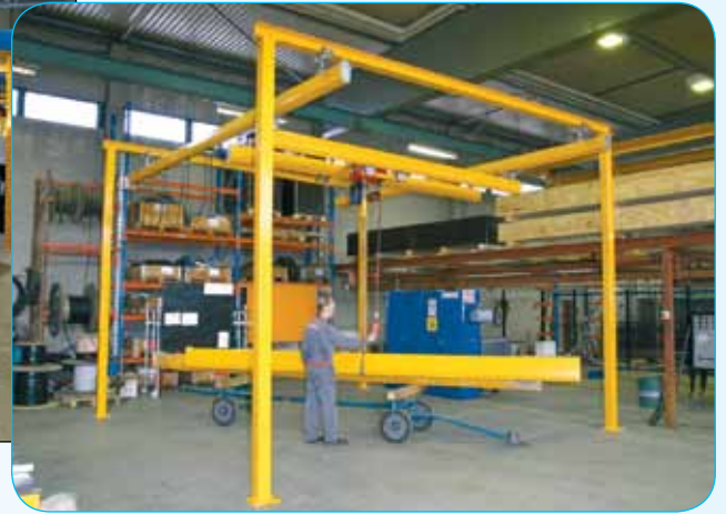
Freestanding-construction as standard with equally short delivery times as cranes.
