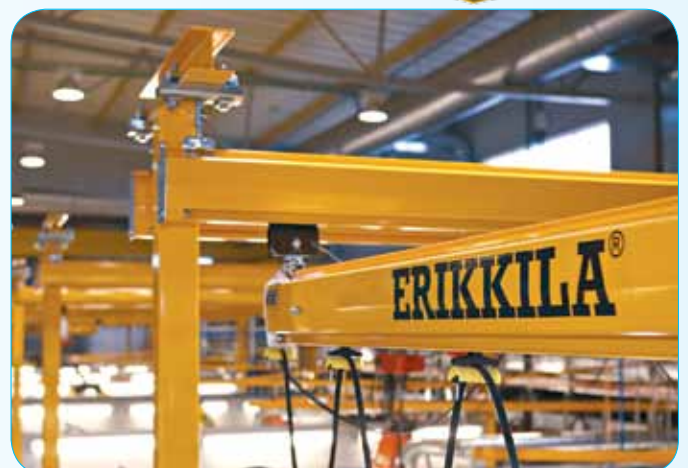
Optimised profiles enable longer suspension distances.
